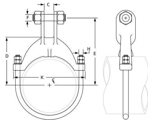
**Fig. 224: Dimensions (in) • Loads (lbs) • Weight (lbs)**
